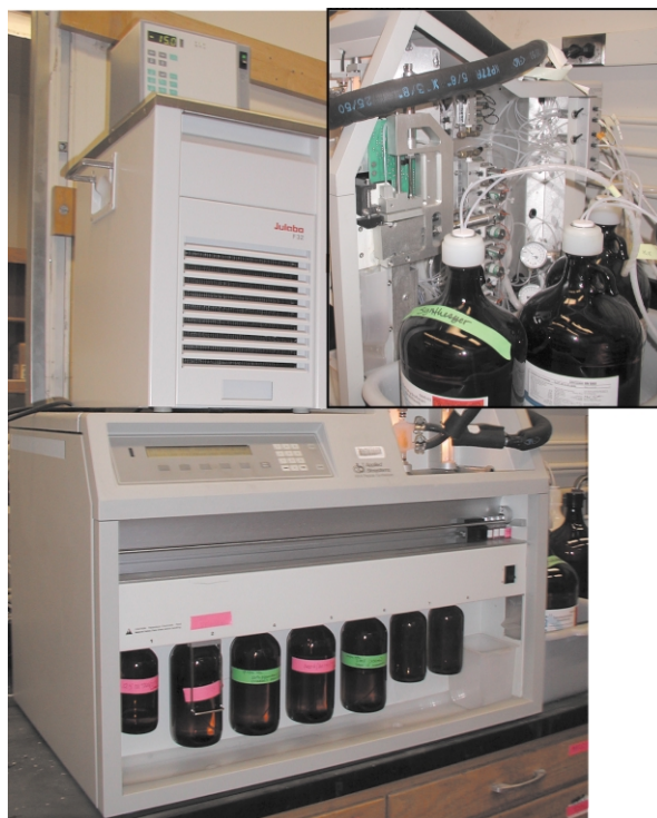
Fig. 2 The first automated oligosaccharide synthesizer based on an ABI 433 peptide synthesizer.
