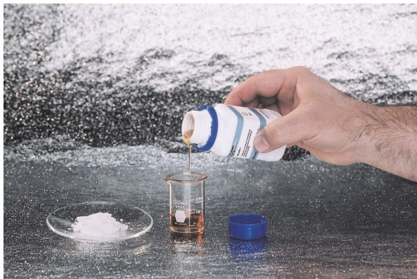
Fig. 4 Not all ionic liquids are actually “liquid” at room temperature. Left is methyltri-n-butylammonium docusate, with a mp around 40 °C. Right is an RTIL (room temperature ionic liquid) 1-butyl-3-methyl imidazolium diethyleneglycolmonomethylethersulfate. Note that some ionic liquids are colorless, while others are pale yellow to orange in colour.
