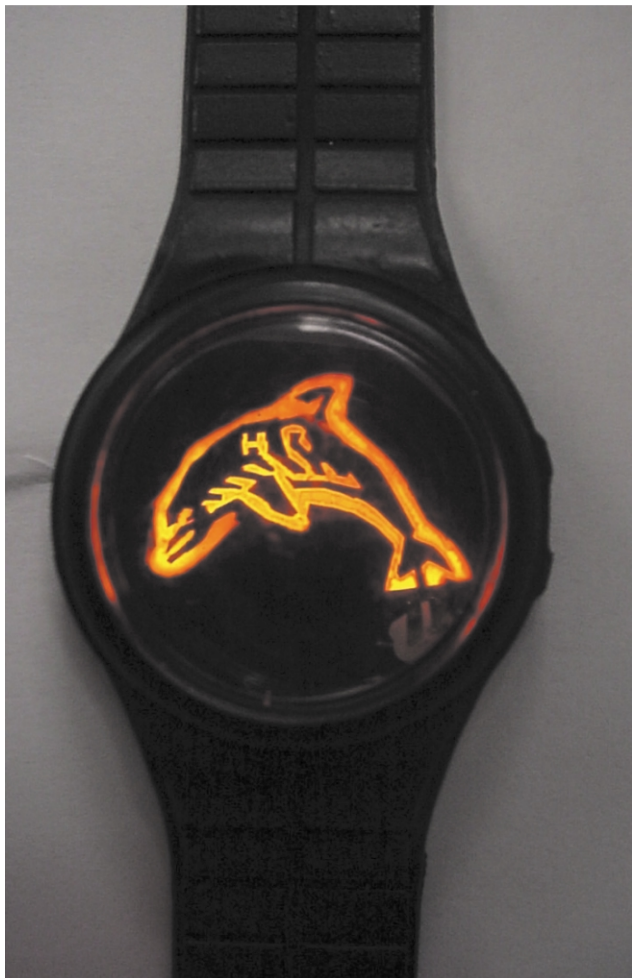
Fig. 8 Electroluminescent device based on [\text{Ru}(\text{bpy})_3]^{2+} . Photo courtesy of Professor Michael Rubner, MIT.
