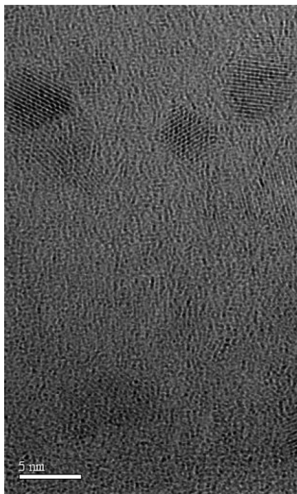
Fig. 2 Bright field HRTEM images of n -butyl capped germanium nanocrystals (10 min growth period) on an ultra thin carbon grid.
