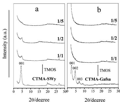
**Fig. 2** XRD patterns of silica–organoclay mesophases prepared from TMOS and CTMA-SWy (a) and CTMA-Gafsa (b) organoclays, for different organoclay/TMOS w/w ratios (1/1, 1/2 and 1/5).
