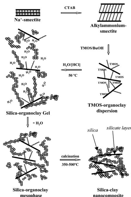
Fig. 1 Scheme showing the steps in the procedure of synthesis of the silica–clay nanocomposites.
