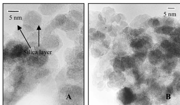
Fig. 1 TEM photographs of silica encapsulated nano-composites.
