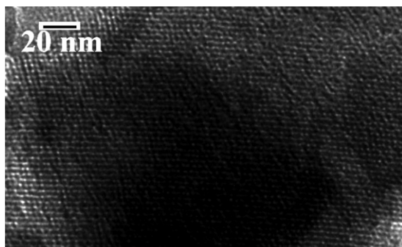
Fig. 3 A representative TEM image of the powders after calcination in nitrogen at 900 °C for 4 h. (taken along the [110] direction)
