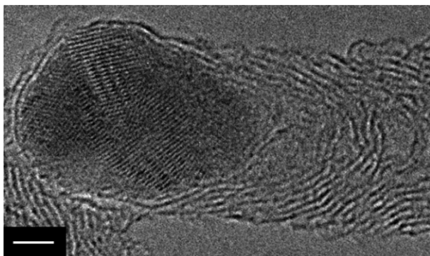
Fig. 3 HRTEM image of an individual CNF from the sample shown in Fig. 2. Scale bar is 2 nm.
