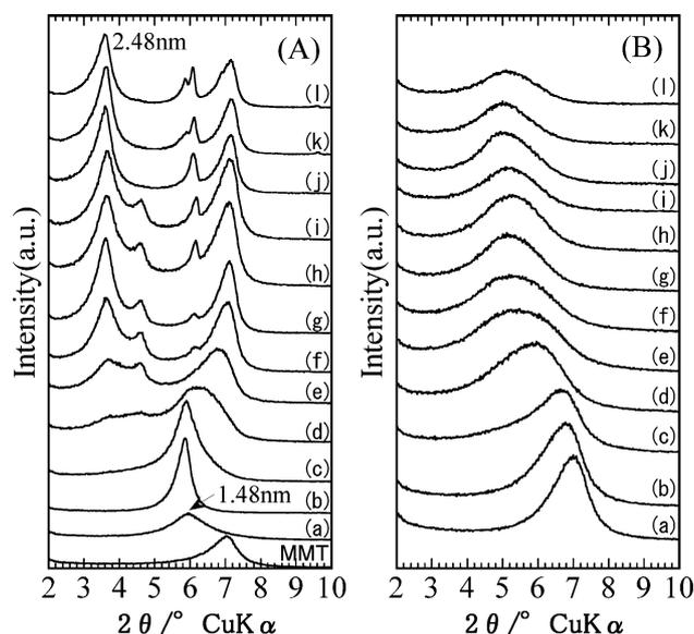
Fig. 1 X-ray diffraction patterns of AF-intercalated MMT with various amounts of added AF (A) before and (B) after polymerization, together with sodium MMT after grinding for 10 min. (a) 1.15, (b) 2.3, (c) 3.45, (d) 4.6, (e) 5.75, (f) 6.9, (g) 8.05, (h) 9.2, (i) 10.35, (j) 11.5, (k) 13.8 and (l) 17.25 (mmol/1g of MMT).
