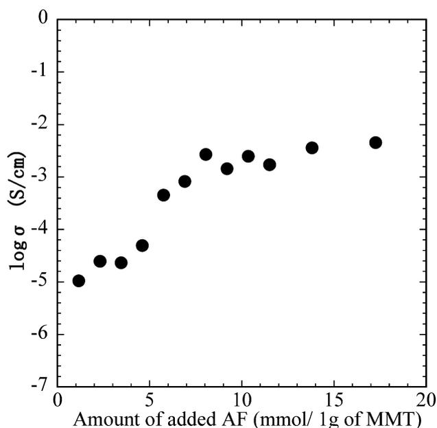
Fig. 3 Conductivities of PANI–MMT nanocomposites.
