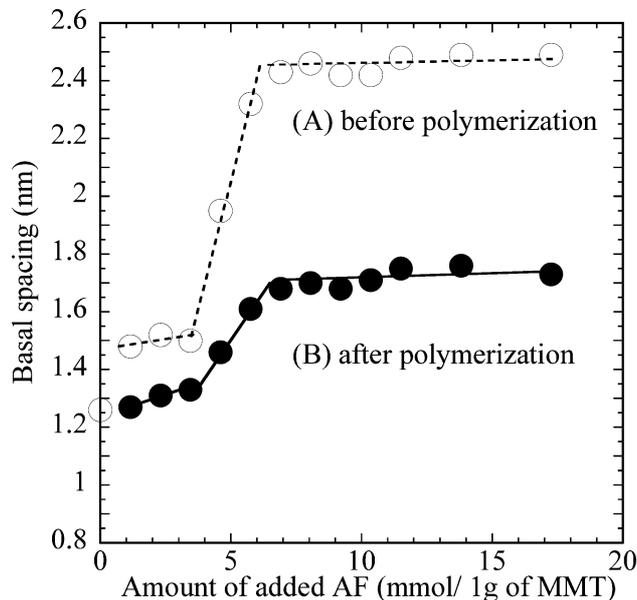
Fig. 2 Plots of the basal spacing versus the amount of added AF, (A) before (○) and (B) after (●) polymerization.
