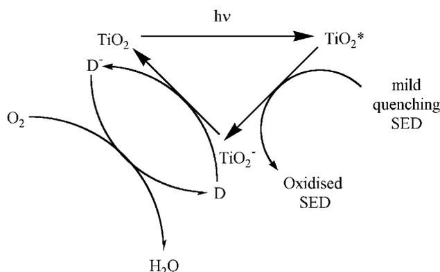
**Fig. 2** Schematic illustration of the key processes involved in the UV-activation and subsequent response towards oxygen of a TiO<sub>2</sub>-MB-TEOA-HEC indicator.
