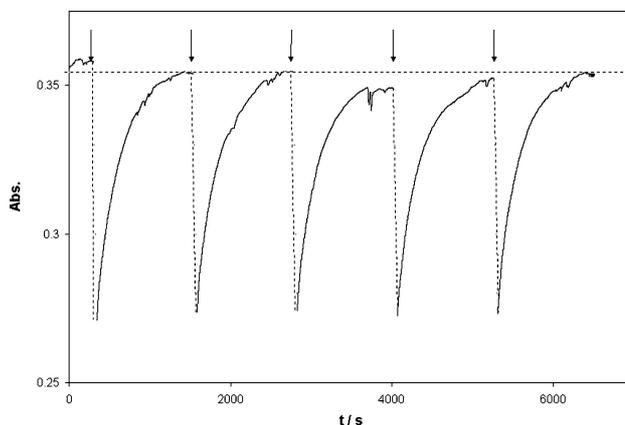
**Fig. 3** Absorbance (610 nm) versus time profile recorded for a typical TiO<sub>2</sub>-MB-TEOA-HEC indicator upon repeated exposure (indicated by ↓) to 2 min of UV-A light (100 W BLB) under ambient aerobic conditions.
