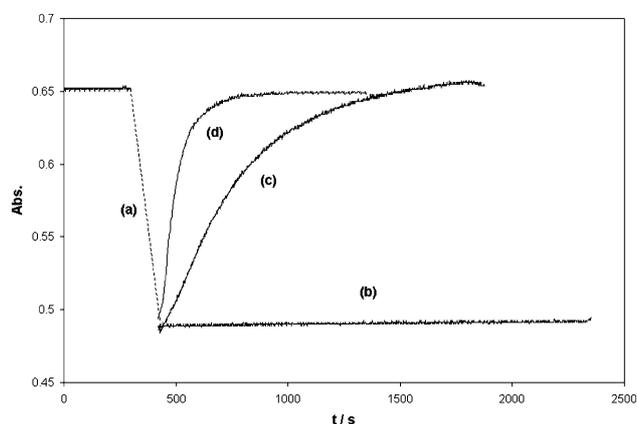
**Fig. 1** Variation in the absorbance (610 nm) of a typical TiO<sub>2</sub>-MB-TEOA-HEC indicator as a function of time upon (a) illumination for 2.5 min with UV-A light (100 W BLB) in a gaseous environment of (b) nitrogen (where the photobleached state persists indefinitely), (c) air and (d) oxygen (where the film recovers its colour with increasing rate).
