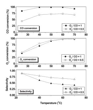
Fig. 2 Preferential oxidation of CO over 0.2 g Au/TiO<sub>2</sub> at different temperatures. Feed composition:  $CO/O_2/H_2/CO_2/H_2O/N_2 = 1/0.5$  or 1/50/15/3/balance (vol%), total flow rate = 110 ml min<sup>-1</sup>.
