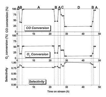
**Fig. 1** Preferential oxidation of CO over 0.04 g Au/TiO<sub>2</sub> versus time on stream at 25 °C. Feed composition: CO/O<sub>2</sub>/H<sub>2</sub>/CO<sub>2</sub>/H<sub>2</sub>O/N<sub>2</sub> = 1/1/50/0 or 15/0 or 3/balance (vol%), total flow rate = 110 ml min<sup>-1</sup>. **A.** without CO<sub>2</sub> and H<sub>2</sub>O in the feed. **B.** with 3% H<sub>2</sub>O in the feed. **C.** with 15% CO<sub>2</sub> in the feed. **D.** with 3% H<sub>2</sub>O and 15% CO<sub>2</sub> in the feed.
