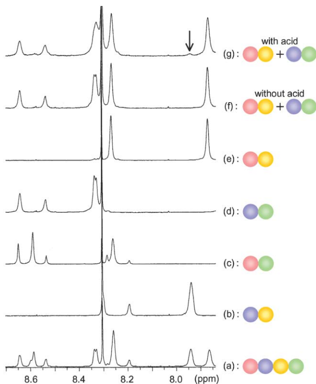
Fig. 4 Part of the ^1\text{H} NMR spectra of (a) the random copolymer P5 , the homopolymers (b) P4 , (c) P3 , (d) P2 , (e) P1 , and the polymer blends (f) without acid B2 and (g) with acid B1 in \text{DMSO-d}_6 (ca. 8 \text{ mg ml}^{-1} ) showing the C–H proton signals of the acylhydrazone functions (signal of \text{CHCl}_3 remaining in the polymers at around 8.32 ppm).
