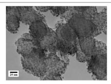
Simple and controllable synthesis of highly dispersed Pt-Ru/C catalysts by a two-step spray pyrolysis process
