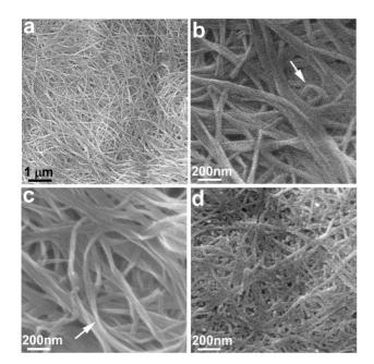
Fig. 1 SEM images of BC membranes (a, b), BC-titania hybrid membranes (c), and titania networks templated by BC membranes (d). Arrows indicate the twisted structure of ribbon-like nanofibers.
