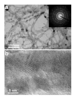
Fig. 2 TEM (a) and HRTEM (b) images of titania nanowires constituting networks templated by BC membranes. Inset shows the corresponding ED pattern.
