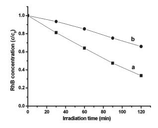
Fig. 4 Photodegradation of Rhodamine B monitored as the normalized concentration change *versus* irradiation time in the presence of titania networks templated by BC membranes (a) and eggshell membranes (b).
