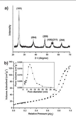
**Fig. 3** XRD pattern (a) and nitrogen adsorption–desorption isotherms (b) of titania networks templated by BC membranes. Inset shows the poresize distribution determined from the desorption branch.
