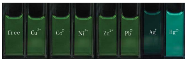
Fig. 1 The fluorescence emission response of 1 ( 3 \times 10^{-6} M) on addition of 3 \times 10^{-6} M cations in the form of acetate salts in aqueous solution of acetonitrile excited at 254 nm using UV lamp. Left to right: free metal, \text{Cu}^{2+} , \text{Co}^{2+} , \text{Ni}^{2+} , \text{Zn}^{2+} , \text{Pb}^{2+} , \text{Ag}^+ , \text{Hg}^{2+} .
