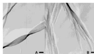
Fig. 9 Structure of bisurea appended thiophene oligomers and electron micrographs of the lamellar fibers of 17 (A) and 18 (B). (Reprinted with permission from Ref. 56. Copyright 1999 Wiley-VCH.)
