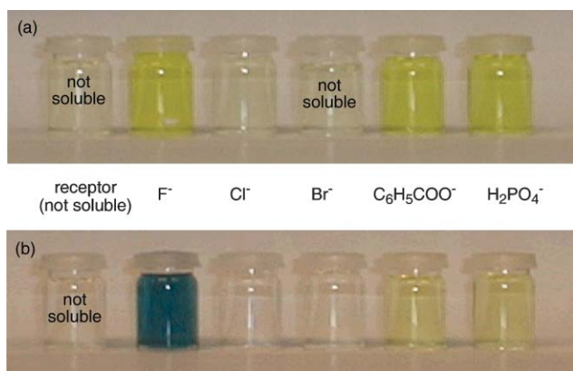
Fig. 11 Solutions of (a) receptor 15 and (b) receptor 16 (2 mM) in acetonitrile with various anionic guests (added as their tetrabutylammonium salt at a concentration of 20 mM). In the absence of an anion, the receptors are not soluble in this solvent but are solubilised upon addition of the anion (with the exception of receptor 2 and bromide).
