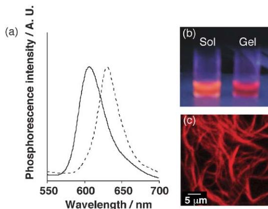
**Fig. 5** Luminescence spectra of the **1Pt** + *p*-xylene gel (dashed) and **1Pt** + 1,1,2,2-tetrachloroethane solution (solid), [**1Pt**] = 2.0 mg ml<sup>-1</sup>; excited at 490 nm for the gel and at 460 nm for the sol, (b) photograph of the **1Pt** gel and sol under UV light (365 nm), (c) CLSM image of the **1Pt** + *p*-xylene gel, [**1Pt**] = 2.0 mg ml<sup>-1</sup>.
