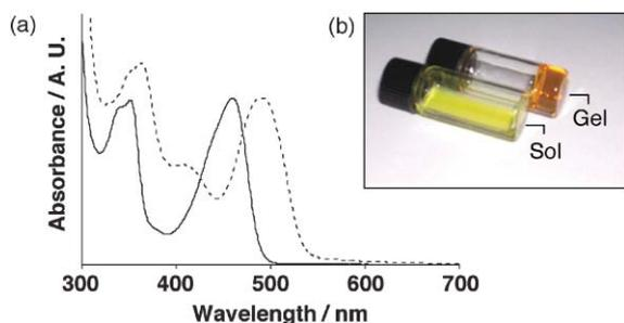
**Fig. 2** (a) Absorption spectra of the **1Pt** + *p*-xylene gel (dashed) and the **1Pt** + 1,1,2,2-tetrachloroethane solution (solid), [**1Pt**] = 10 mg ml<sup>-1</sup>, and (b) photograph of the **1Pt** + *p*-xylene gel and its heated solution (sol).
