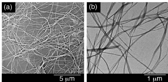
**Fig. 1** (a) SEM and (b) TEM images of the **1Pt** + 1-butanol gel, [**1Pt**] = 2.0 mg ml<sup>-1</sup>.
