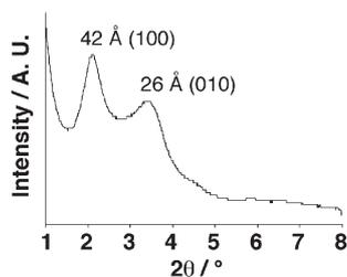
**Fig. 3** Powder XRD diagram of the xerogel prepared from the **1Pt** + benzene gel, [**1Pt**] = 200 mg ml<sup>-1</sup>.
