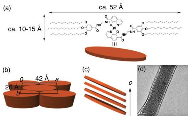
**Fig. 4** (a) Molecular scales of **1Pt**, (b) proposed packing model of **1Pt** in the gel tissues, (c) tilted arrangement of **1Pt** along the *c* axis, (d) HR-TEM image of the **1Pt** + *p*-xylene gel, [**1Pt**] = 2.0 mg ml<sup>-1</sup>.
