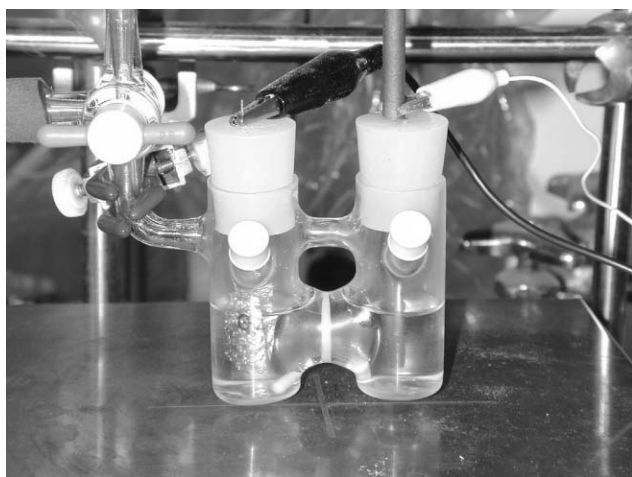
Fig. 5 An H-type electrochemical cell for the "cation pool" method.
