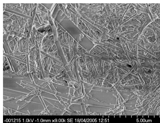
Fig. 4 SEM image of metallo gel derived from 1 and copper(II) nitrate.
