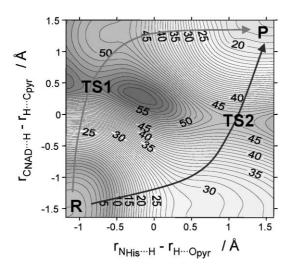
**Fig. 1** PES 1: QM/MM contours (kcal mol<sup>-1</sup>) for pyruvate (R) to lactate (P) LDH-catalyzed reaction. The protonation state of the ionizable groups in protein were calculated at pH = 7 using the standard  $pK_a$  values in aqueous solution.
