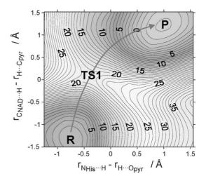
Fig. 3 PES 3: QM/MM contours (kcal  $mol^{-1}$ ) for pyruvate (R) to lactate (P) LDH-catalyzed reaction, with MP2/6-31G(d,p) corrections. Protonation states of ionizable groups in protein are as for PES 2.
