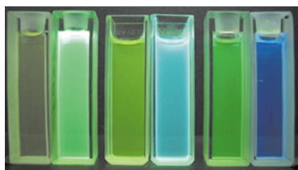
Fig. 1 Photograph of 2 and 4 solutions under UV irradiation (365 nm). From left to right: 2 , 4 in DMF, 2 , 4 in THF, 2 , 4 in hexane (ca. 10 -6 M).
