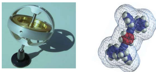
Fig. 1 (Left) A gyroscope is a device consisting of a spinning mass, or rotor (gold), with a spinning axis positioned through the center of the mass, and mounted within a rigid frame (silver). (Right) Analogous to the macroscopic object, molecular gyroscope 1 contains a phenylene rotor (red) with an alkyne axle and shielding groups that encapsulate it (blue).
