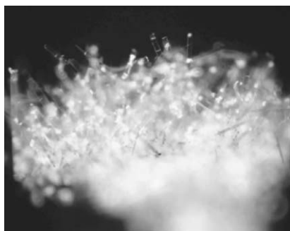
Fig. 3 PL microscopic image of ZnS nanobelts excited by light with a wavelength of 380 nm.
