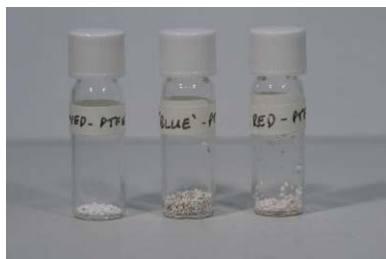
Fig. 4 PTFE (L to R): unmodified; modified with precursor 2d followed by diazonium salt 6 ; modified with precursor 2d followed by diazonium salt 5 .
