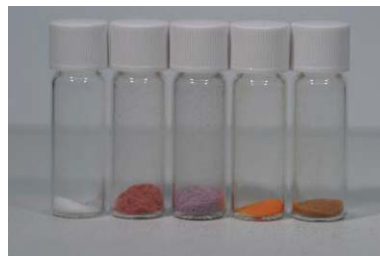
Fig. 2 Silica (L to R): unmodified; modified with precursor 2d followed by diazonium salt 5 ; modified with precursor 2d followed by coupling with diazonium salt 6 under alkaline conditions; modified with precursor 2d followed by diazonium salt 6 with acid wash; modified with precursor 2d followed by diazonium salt 7 .
