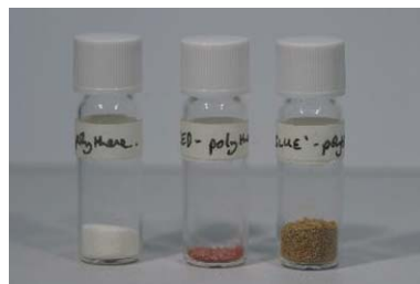
Fig. 3 Polythene (L to R): unmodified; modified with precursor 2d followed by diazonium salt 5 ; modified with precursor 2d followed by diazonium salt 6 .
