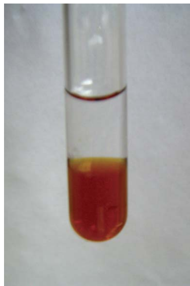
Scheme 2 Immobilized Ir-(P-Phos) catalyst in hexane/DMPEG biphasic system (lower DMPEG phase).
