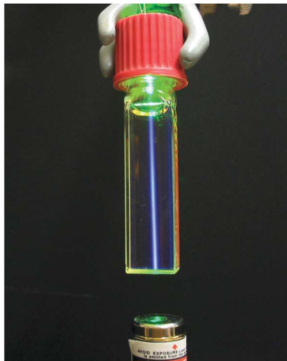
Fig. 3 Digital photograph of upconverted fluorescence produced in 4 : 1 toluene- \text{CH}_3\text{CN} solutions of [\text{Ru}(\text{dmb})_3]^{2+} ( 1.4 \times 10^{-4} M) and DPA (filtered saturated solution). Excitation by a commercial green laser pointer ( \lambda_{\text{ex}} = 532 nm, <5 mW peak power).
