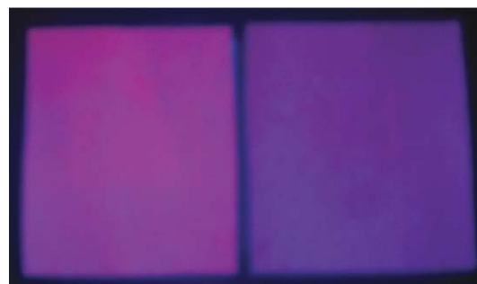
Fig. 3 Thin films of POT (left) and POT with 3-octadecylthiophene (right, X_p = 0.50 ) irradiated by UV light (365 nm).
