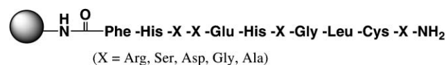
Fig. 1 Combinatorial library of 625 (5 4 ) peptides synthesized by the split-and-pool method with the X positions varied over the five AAs given in parentheses.
