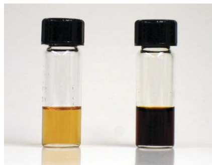
Fig. 1 Photograph of the [BMIM][Tf 2 N] IL mixture after the reaction (left vial) and the dispersion of nanoparticles in hexane (right vial). The reaction was conducted using silver trifluoroacetate and oleic acid at 200 °C. The reaction time was 40 min.
