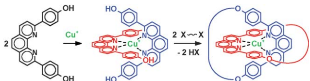
Fig. 2 Controlled synthesis of a [2]catenane; prearrangement of the linear precursors via coordination to a metal cation as template. 13
