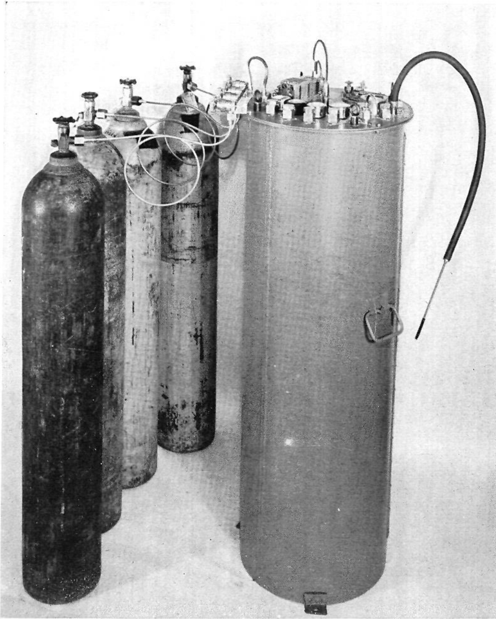
FIG. 9. Pump unit with rotating column for producing either liquefied oxygen or high-pressure gaseous oxygen.
