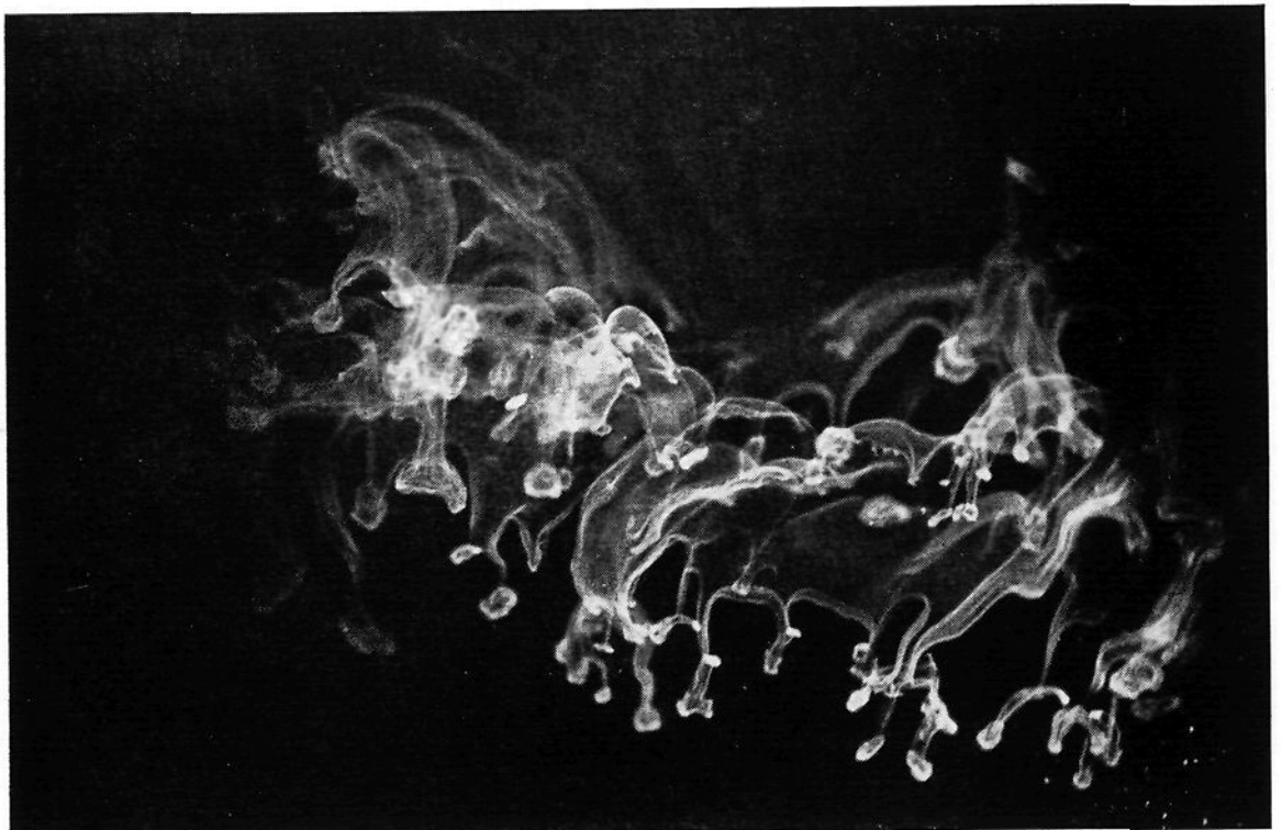
FIG. 8. Trail of ice crystals produced in cold chamber by seeding with needle cooled below -39^{\circ}\text{C} .
