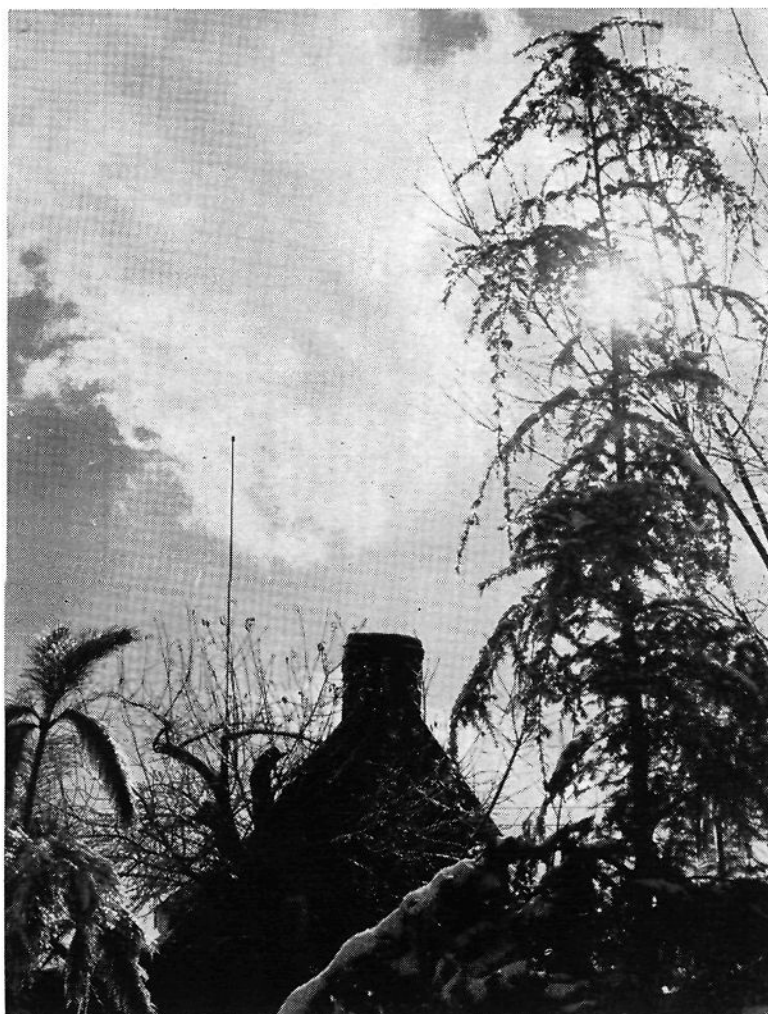
FIG. 1. Satisfactory exposure for point collector to record atmospheric electricity
