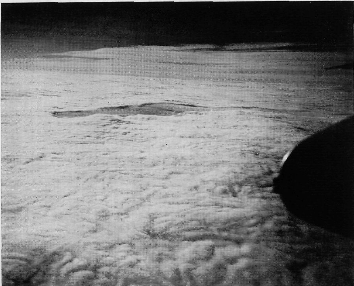
FIG. 22. Photograph of modified stratus cloud seeded at rate of 1 lb. per mile. The modified area which appears dark is 15 miles long and 2 miles wide.
