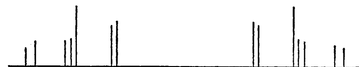
FIG. 16. Experimental and theoretical spectra for the protons in ethylene monothiocarbonate. The experimental trace is that of the pure liquid at room temperature and 40 Mc./sec.
