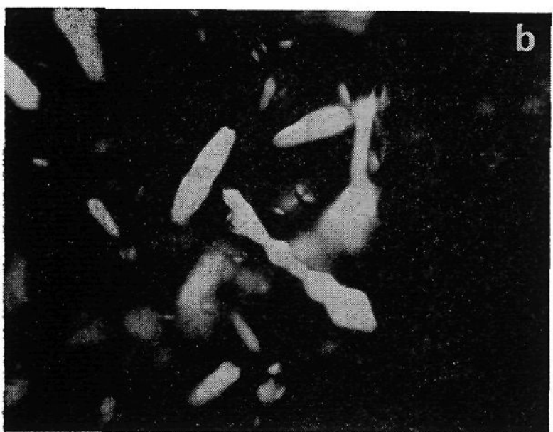
Figure 12.—Batonnets of the M_1 phase precipitated after peripheral evaporation (section IV.B.7) of a 30% isotropic aqueous solution of sodium caprylate for several days at 20^\circ ( \times 65 , crossed polars). The interior markings derive from interference colors. (b) Batonnets of the G phase precipitated at the S-G phase boundary in the N,N,N-trimethylaminododecanoimide-water system (section II.B.2): sample prepared by peripheral hydration of supercooled liquid imide at 20% relative humidity at 20^\circ ; the batonnets successively redissolve and reprecipitate when illumination of slide is cyclicly increased and diminished ( \times 150 , crossed polars).
