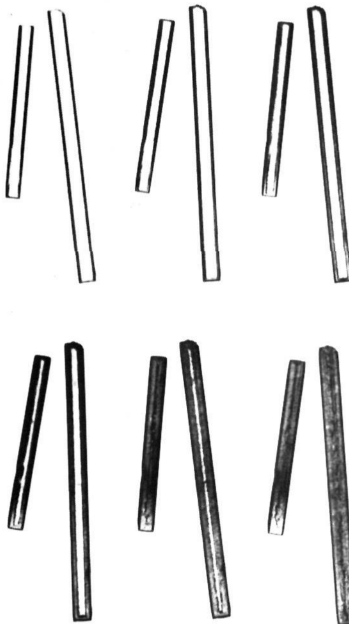
Figure 7. Pair of centrosymmetric crystals of p -chlorobenzoic anhydride (7b) undergoing reaction with ammonia gas. Regions where reaction has occurred appear dark because the microcrystalline products scatter the transmitted light. (Reprinted with permission from R. S. Miller, D. Y. Curtin, and I. C. Paul, J. Am. Chem. Soc. , 94 , 5778 (1972). Copyright 1972, American Chemical Society.)
