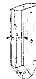
Figure 1. Pictures from P. Groth's Chemische Kristallographie . Upper drawing: centrosymmetric crystals of acetanilide (1), space group Pbca (class mmm ). Lower drawing, a polar crystal of p -chloroacetanilide (2), space group Pna2 1 (class mm2 ).
