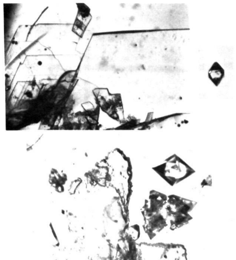
Figure 23. (Upper left) A thin plate of the low-temperature achiral form of binaphthyl (24). (Upper right) A tetragonal bipyramid of the high-temperature form. (Below) A plate of the low-temperature form which has been heated. The product crystals can be seen growing at the right side of the photograph. (Reproduced with permission from ref 54. Copyright 1980, American Chemical Society.)
