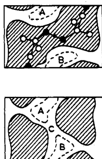
Figure 35. D_i (the fraction of the occupied space) map of azobis(isobutyronitrile) before (a) and after (b) elimination of nitrogen.
