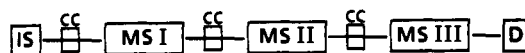
Figure 3. Schematic drawing of a multisector mass spectrometer, consisting of an ion source (IS), three sectors (MS I-III), which can be either magnetic or electrostatic analysers, several collision cells (CC), and a detector (D).
