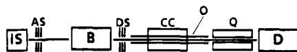
Figure 2. Schematic drawing of a guided ion-beam instrument, consisting of ion source (IS), acceleration (AS) and deceleration (DS) stage, magnetic sector (B), octopole ion guide (O), collision chamber (CC), quadrupole mass filter (Q), and detector (D).
