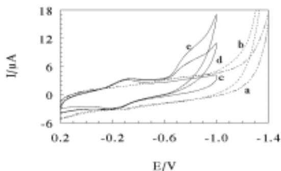
(a) DHP-PDDA film; (b) DHP-PDDA film in buffers containing  $0.1\text{ mmol L}^{-1}\text{ NO}_2^-$ ; (c) Hb-DHP-PDDA film; (d) Hb-DHP-PDDA film in buffers containing  $0.1\text{ mmol L}^{-1}\text{ NO}_2^-$ ; (e) Hb-DHP-PDDA film in buffers containing  $0.2\text{ mmol L}^{-1}\text{ NO}_2^-$ .
