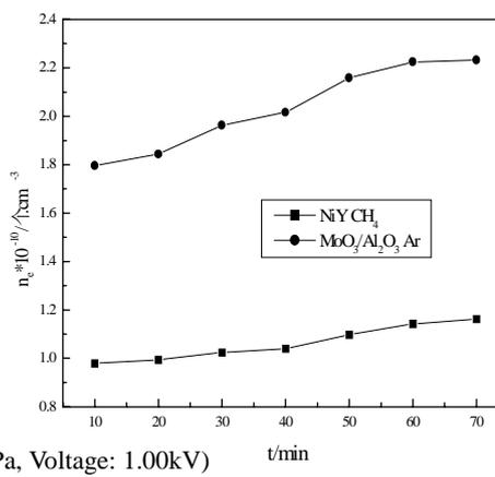
**Figure 1** shows that the electron temperature over NiY catalysts in methane and over MoO<sub>3</sub>/Al<sub>2</sub>O<sub>3</sub> catalysts in argon increases with prolonging the cold plasma treatment time. **Figure 2** indicates that the electron density also increases with prolonging the cold plasma treatment time.
