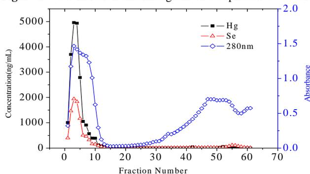
The supernatant extracted from the liver powder by alkaline protease in the presence of 1% SDS was subjected to the column (1.2×60 cm). Eluent: 0.1 mol/L  $\text{NH}_4\text{Ac-NH}_3$  (pH 9)
