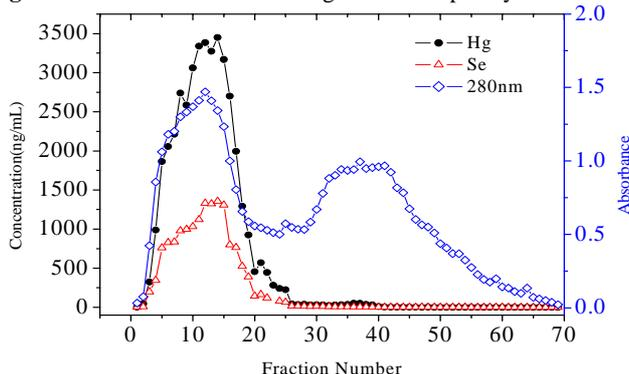
The fractions of void volume on Sephadex G-75 were lyophilized and the mixture of it reacted with DDT and DDTC was subjected to the column (1.2×60 cm). Eluent: 0.1 mol/L  $\text{NH}_4\text{Ac-NH}_3$  (pH 9)
