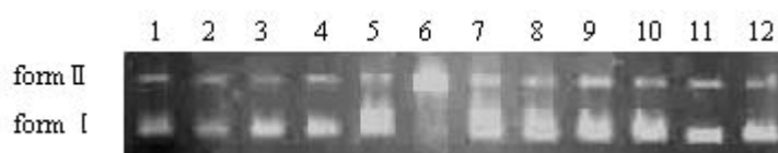
Figure 2 Cleavage of DNA(0.325 mmol/L) by Cu(II) complex (1 mmol/L) as a function of pH.
