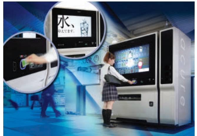
Image 1: Mutual capacitive touch technology is very well suited to touchscreen applications requiring multitouch functionality, as each cell within the conductive matrix is capable of registering a touch. (All images courtesy of Zytronic)
