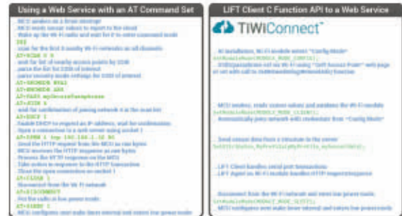
Figure 2. Comparison of an ASCII Command Set approach and TiWiConnect’s LIFT Client approach for a common device-to-cloud Wi-Fi transaction.
