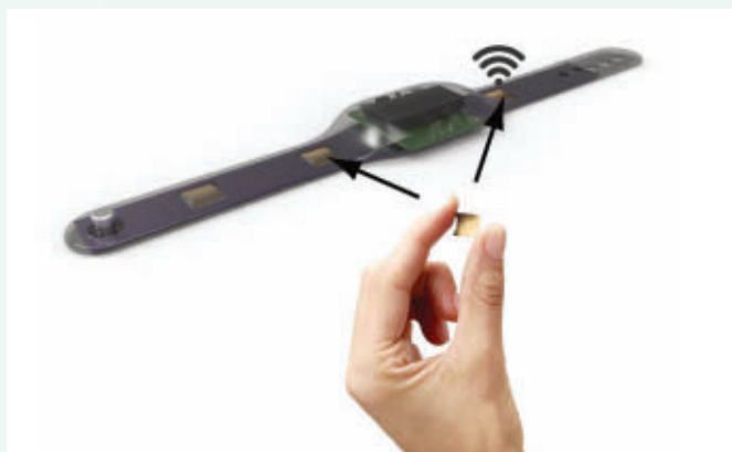
Figure 1. This wearable device features haptic actuators that are buried in the band. (Photo courtesy Novasentis.)
