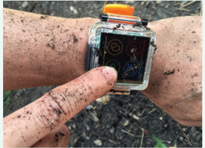
Figure 2. Touch technology that can work with gloves, sweaty fingers and even in dirt and sand. (Photo courtesy UICO).
