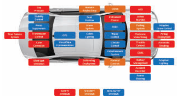
Figure 1: Embedded software powers all major systems of today's automobiles including: engine control, power train, braking and airbags, driver assistance, infotainment and much more. (All figures courtesy of Vector Software).
