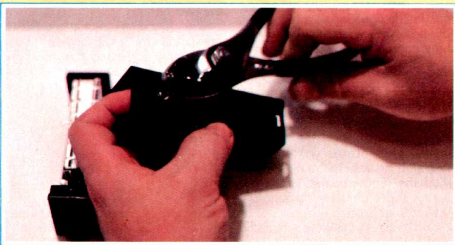
FIGURE 6: After inserting the jack through the newly-made hole, tighten the collar with the pliers and tape the soldered contact.
