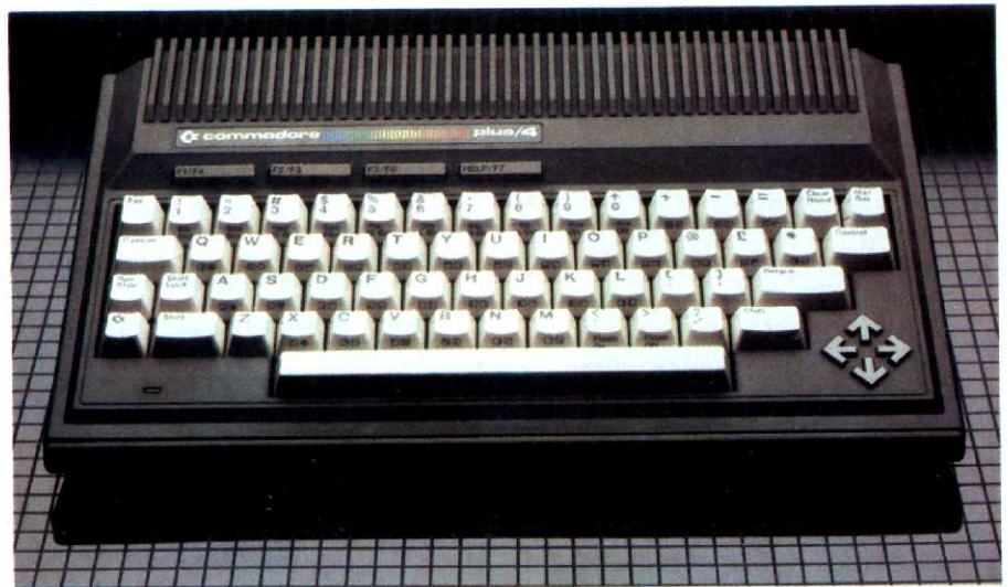
The Plus/4: unlike the C-64, the function keys are above the keyboard, the cursor keys are in a "compass configuration".
