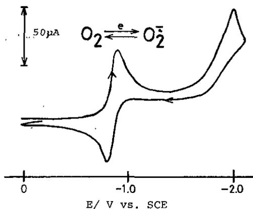
Fig. 1. Cyclic voltammograms of oxygen. electrolyte:  $0.1 \text{ M}$  TEAP/DMF, electrode: HMDE, sweep rate:  $0.1 \text{ Vs}^{-1}$ .
