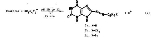
bromo derivatives to form azo compounds as expected.<sup>15</sup> The yields of these azo compounds ranged from 24 to 60%. The absence of the resonance signal of the 8 proton in the NMR spectra confirmed the site of the substitution reaction. The spectroscopic properties of these compounds are presented in Table II. The related nucleoside, xanthosine, does not react with benzenediazonium ion to give an azo compound or the 8 phenylation product.
