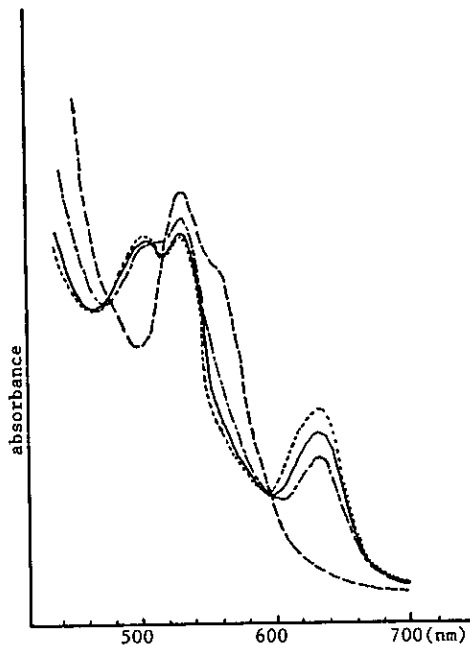
Fig.2 Visible spectra of (6) and (7) with imidazoles in DMF. a,(.....)(6) 1.1 \times 10^{-5} M ; b,(—)(6) 1.1 \times 10^{-5} M , N-tritylimidazole 5.5 \times 10^{-3} M ; c,(---)(6) 1.1 \times 10^{-5} M , imidazole 5.5 \times 10^{-3} M ; d,(-----)(7) 1.1 \times 10^{-5} M , N-tritylimidazole 5.5 \times 10^{-3} M .
