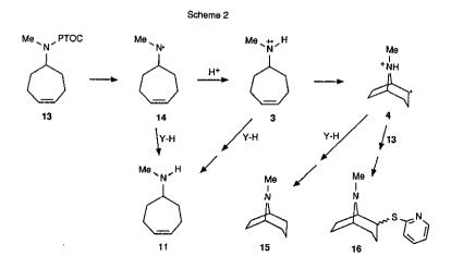
Acetic acid proved to be adequate for protonation of 14 and *tert*-BuSH was an efficient and selective hydrogen atom trapping agent. In visible light initiated reactions similar to those previously described,<sup>2</sup> tropane<sup>10,11</sup> was isolated in 67% yield when *tert*-BuSH was present and sulfides  $16^{10}$  were isolated in 92% yield in the absence of *tert*-BuSH (*exo*-16 : *endo*-16 = 15 : 1).
